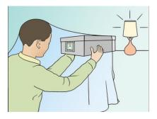
A pinhole camera consists of a box or tube with a translucent screen at one end and a tiny hole (the pinhole) made in the other end.
